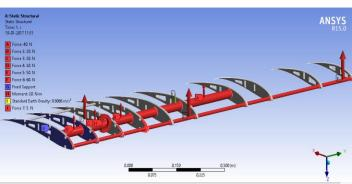
Fig.18 Force application on the wing
