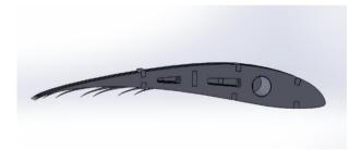
Fig.12 Internal structure of the wing (Top View)
