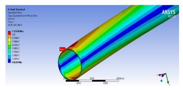
Fig.21 Equivalent Von-mises stress contours in spar
