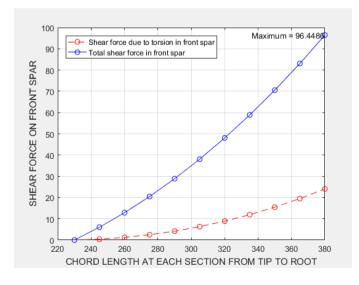
Fig.9 Shear Force due to torsion; Total shear in front spar
