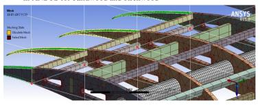
Fig.14 Failed & Obsolete Mesh (1st attempt)
