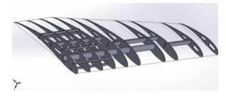
Fig.11 Internal structure of the wing (Isometric View)
